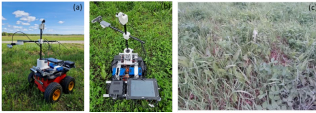
Figure 1. Frontal (a) and superior (b) photos of the robot in the field trial, and an example of an image acquired by the camera with a viewing angle of 45° (c). Photos: Julianne Oliveira.
